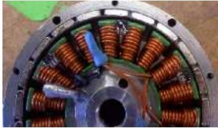
Gambar 2.2 Stator BLDC
