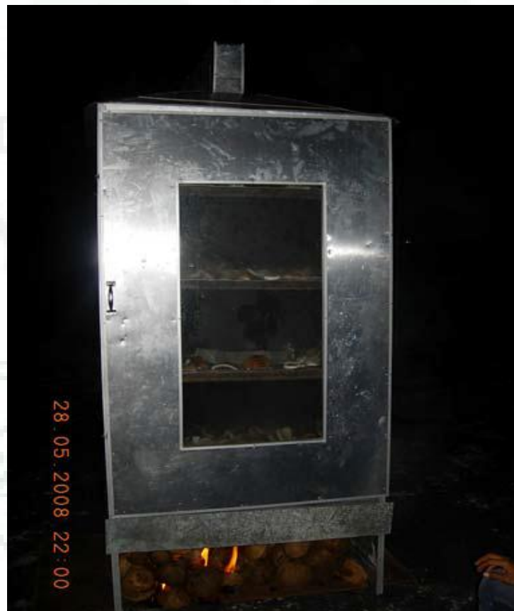
Gambar 2.gambar oven kopra bak pasir perata panas
