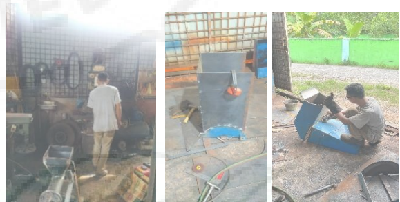
Gambar 8. Fabrikasi Mesin Pencacah Plastik di Workshop CV Star Umroh Engineering.
