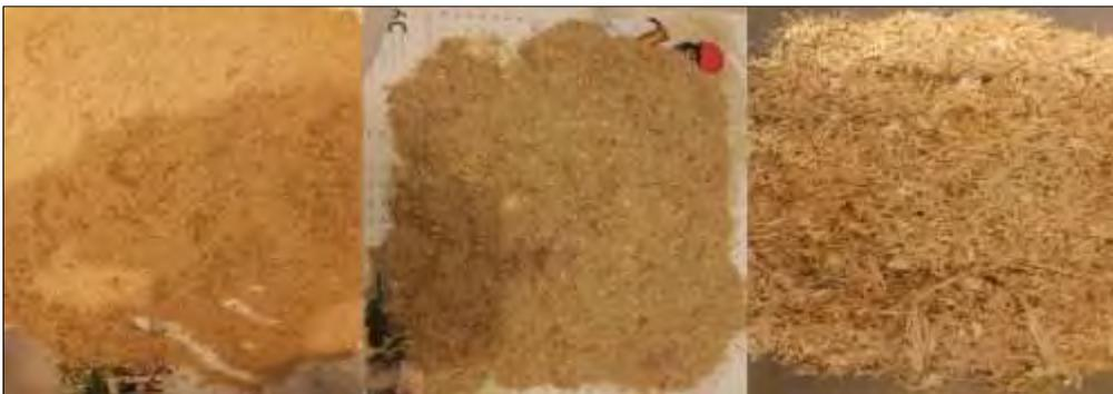
**Figure 2.** Variations of the oil palm trunk fibers used for the manufacture of test objects
