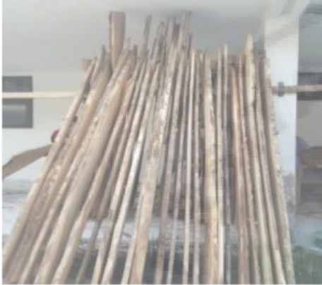
Fig. 7. Drying of teak wood.
