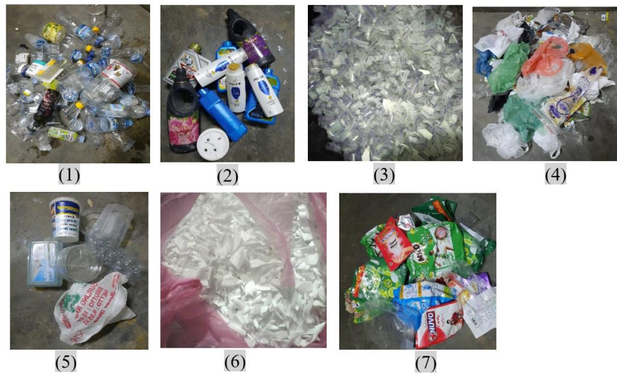
Gambar 1. Jenis plastik bahan penelitian; (1)PET, (2) HDPE, (3) PV, (4) LDPE, (5) PP, (6) PS, dan (7) Other
