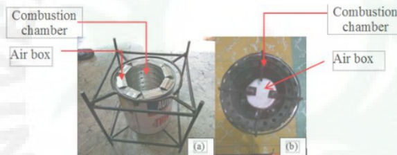
Figure 2: The stoves prototype: (a) External air box, (b). Internal air box
