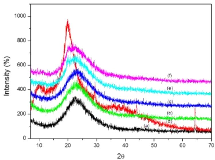
**Fig. 2.** The XRD spectra of: (a) pure silica gel (Sg), (b) pure chitosan (Ch); and for silica-based chitosan biocomposite of: (c) SChC1 (20 mL : 2%), (d) SChC2 (20 mL : 3%), (e) SChC3 (20 mL : 4%), and (f) SChC4 (20 mL : 5%).
