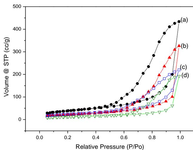
**Fig. 4.** The adsorption-desorption isotherm for silica-based chitosan biocomposites of: (a) SChC1 (20 mL : 2%), (b) SChC2 (20 mL : 3%), (c) SChC3 (20 mL : 4%), and (d) SChC4 (20 mL : 5%). The measurements are made at 77 K.
