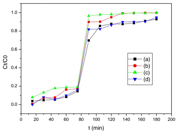
**Fig. 5.** The adsorption capacity toward Cd(II) ion by solid-phase extraction method for biocomposite materials of: (a) SChC1 (20 mL : 2%), (b) SChC2 (20 mL : 3%), (c) SChC3 (20 mL : 4%), and (d) SChC4 (20 mL : 5%). The data are recorded from the proportion of the amount of Cd<sup>2+</sup> after loading ( $C_t$ ) compared to the original Cd<sup>2+</sup> ( $C_0$ ) for 18 minutes.
