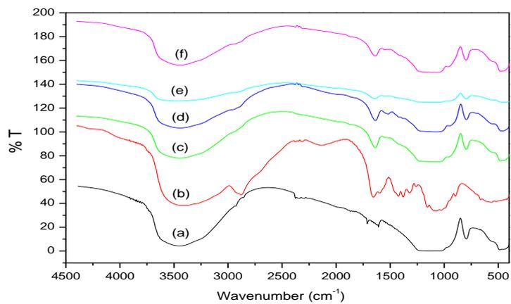
**Fig. 1.** The FTIR spectra of: (a) pure silica gel (Sg), (b) pure chitosan (Ch); and for silica-based chitosan biocomposite of: (c) SChC1 (20 mL : 2%), (d) SChC2 (20 mL : 3%), (e) SChC3 (20 mL : 4%), and (f) SChC4 (20 mL : 5%).
