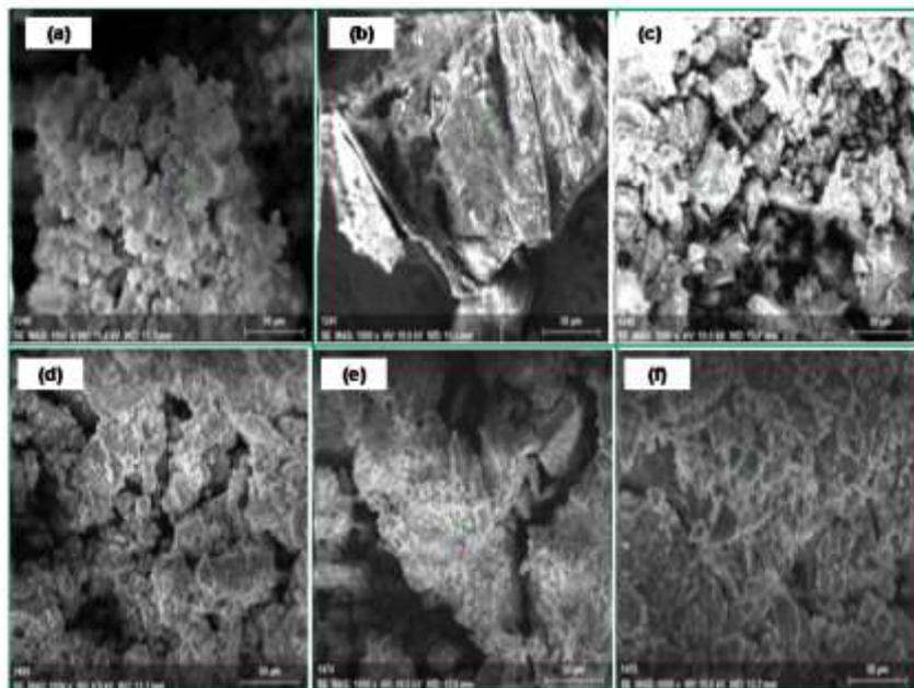
**Fig. 3.** The SEM images of: (a) pure silica gel (Sg), (b) pure chitosan (Ch); and for silica-based chitosan biocomposites of: (c) SChC1 (20 mL : 2%), (d) SChC2 (20 mL : 3%), (e) SChC3 (20 mL : 4%), and (f) SChC4 (20 mL : 5%).
