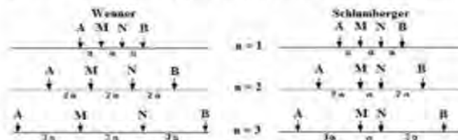
Figure 2. The arrangement of the electrodes in the Wenner and Schlumberger configurations
