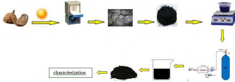
Figure 1: Schematic preparation activated carbon
