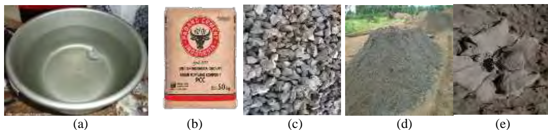
FIGURE 2.1 Material used a) water, b) Portland cement type 1, c) broken stone, d) sand, e) volcanic ash
