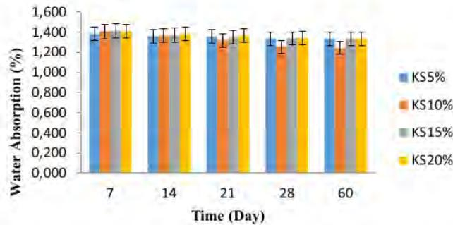
**Figure 3.** Graph Water Absorption Concrete Mixtures with Boyler Ash Palm Oil by Time
