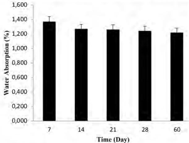
Figure1. Graph Concrete Water Absorption by Time
