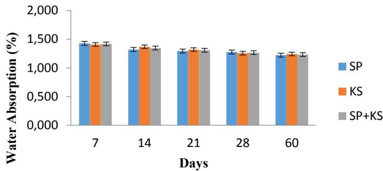
**Figure 11.**Graph Based Absorption Addition In 10% Composition
