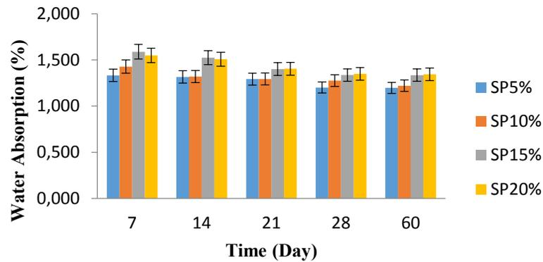
**Figure 2.** Graph Water Absorption Concrete Mixtures with Rice Husk Ash by Time
