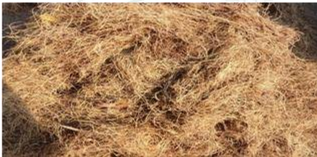
Fig. 9. OPEFB decomposes at 1350 rpm rotation
