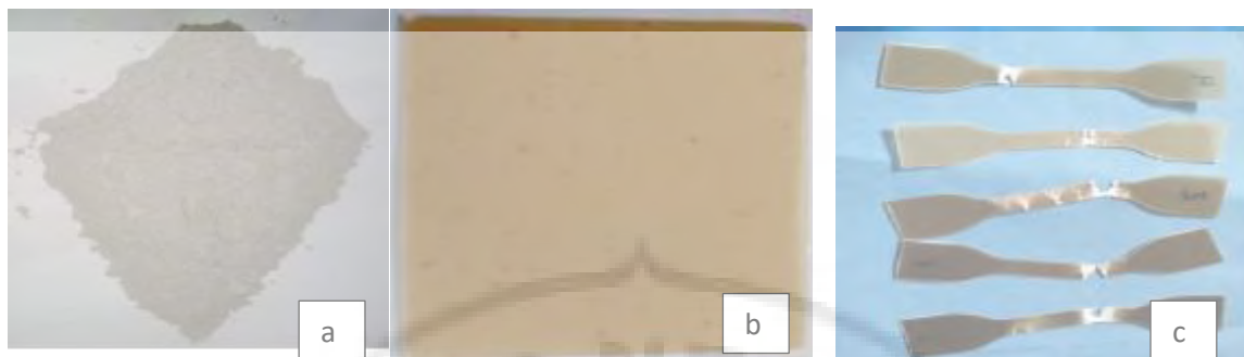
Figure 1. (a) OPEFB nano particles (b) Nano composite TPE (c) Sample test mechanis
