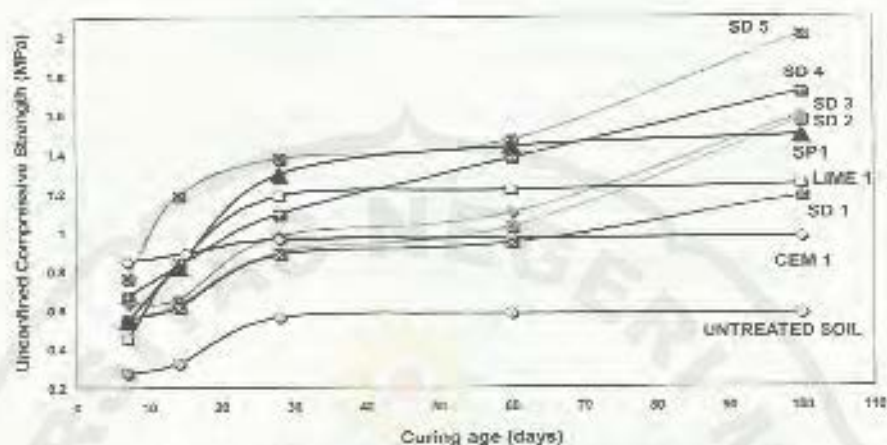
Fig.4. U.C.S development of solidified samples at different curing ages
