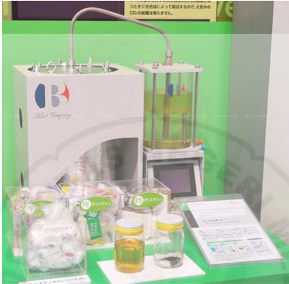
Gambar 10. 1. Mesin pirolisis BLest (Mini Plastic-to-Oil Machine)
