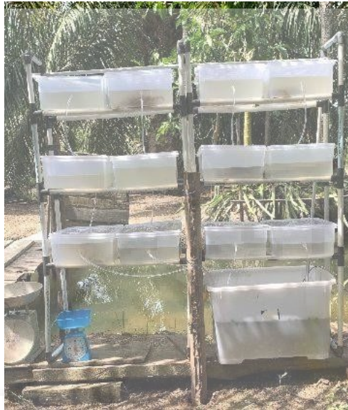
Gambar 4. Contoh sederhana Recirculating Aquaculture System (RAS)
