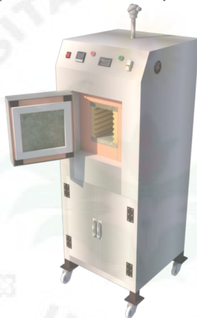
Figures 7. Electric Furnace overview
