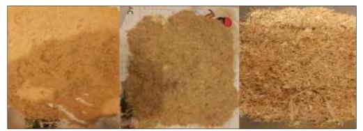
Figure 2. Variations of the oil palm trunk fibers used for the manufacture of test objects
