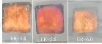
Fig. 3. Flame image captured during operation.
