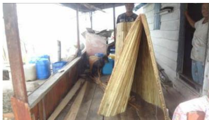
Figure 9. Kajang which functions as a sampan kolek roof
