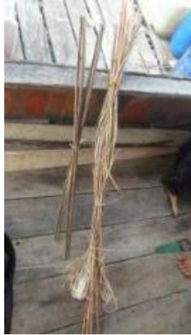
Figure 10. Bone leaves of the coconut tree and rattan leaf bones was used as kajang frames Source: Personal documentation
