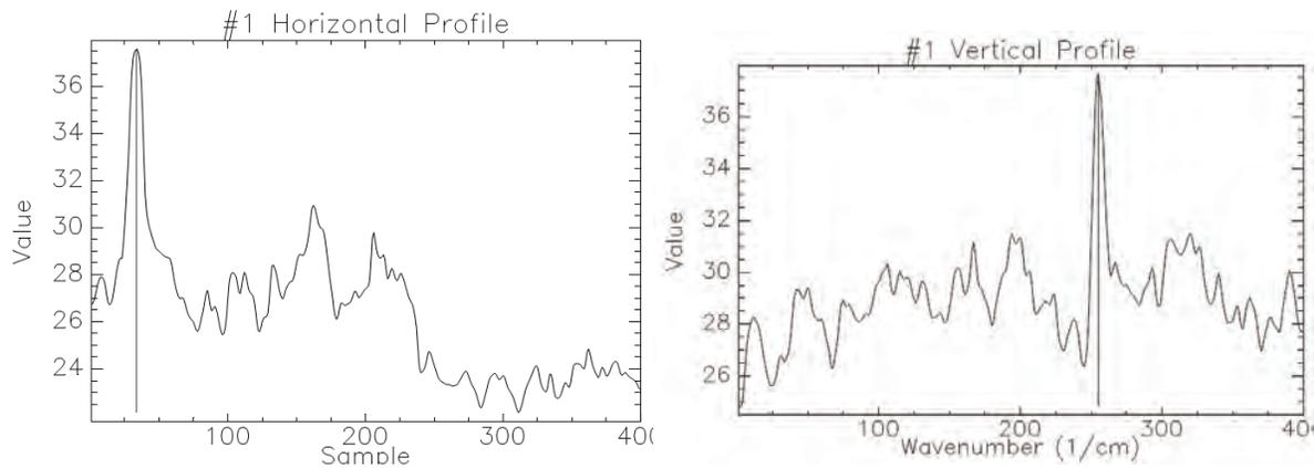
**FIGURE 3.** Horizontal and vertical profile of the predicted point of geothermal resource
