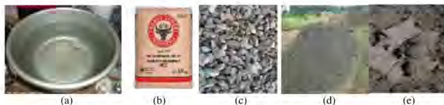
FIGURE 2.1 Material used a) water, b) Portland cement type I, c) broken stone, d) sand, e) volcanic ash
