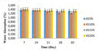
Figure 3. Graph Water Absorption Concrete Mixtures with Boyler Ash Palm Oil by Time
