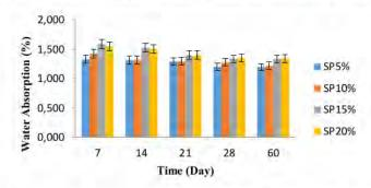
Figure 2. Graph Water Absorption Concrete Mixtures with Rice Husk Ash by Time
