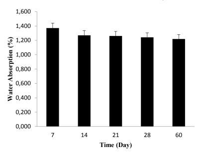
Figure1.Graph Concrete Water Absorption by Time
