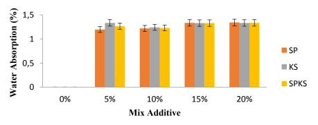
Figure 9. Graph Based Absorption Addition In 60 Days
