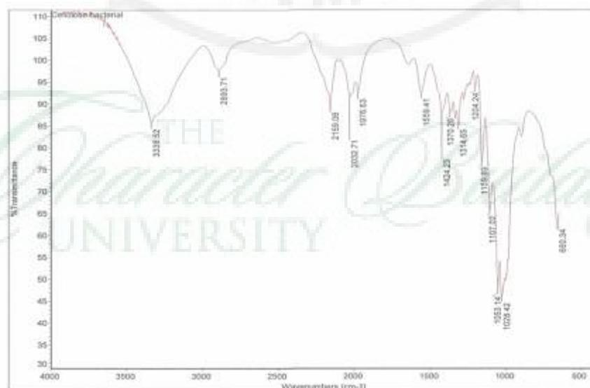
**Figure 5.** FT-IR spectra of BC.
