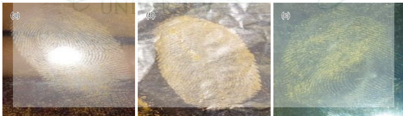
Fig. 1. Latent fingerprint visualization of the dusting method of turmeric powder in: (a) glass preparation; (b) aluminum foil; (c) transparent plastic
