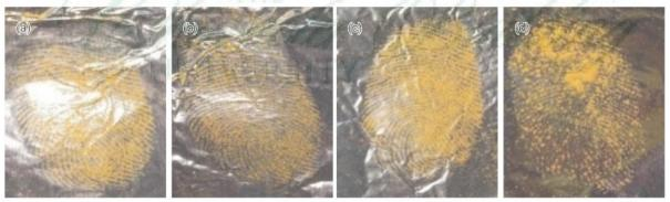
Fig. 10. Comparison of ulnair loop pattern fingerprint visualization on aluminum foil size: (a) 100 mesh oven; (b) 100 mesh sun; (c) 200 mesh oven; (d) 200 mesh sun
