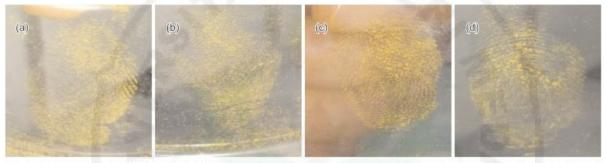
Fig. 8. Comparison of visualization of radial loop pattern fingerprints on plastic cups size: (a) 60 mesh oven; (b) 60 mesh sun; (c) 80 mesh oven; (d) 80 mesh sun
