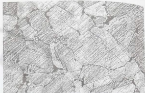
Fig.5 Sample temper 500°C for 30 minutes
