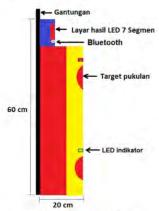
Figure 3: Side View of The Tool
