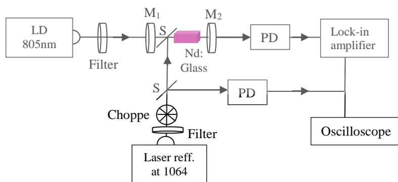
Figure 1. The detailed experiment of laser diode photopumped.
