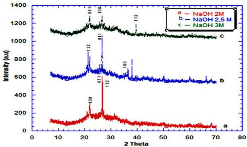
Fig. 2. OPBA diffraction pattern with variation of NaOH solution
