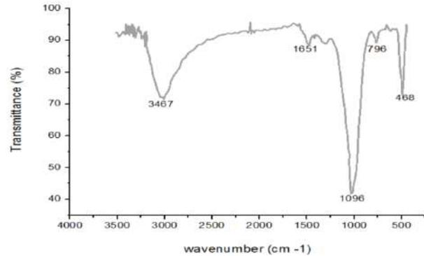
**Figure 4:** FTIR characterization graph**Table 5:** Functional group and Wave Numbers
