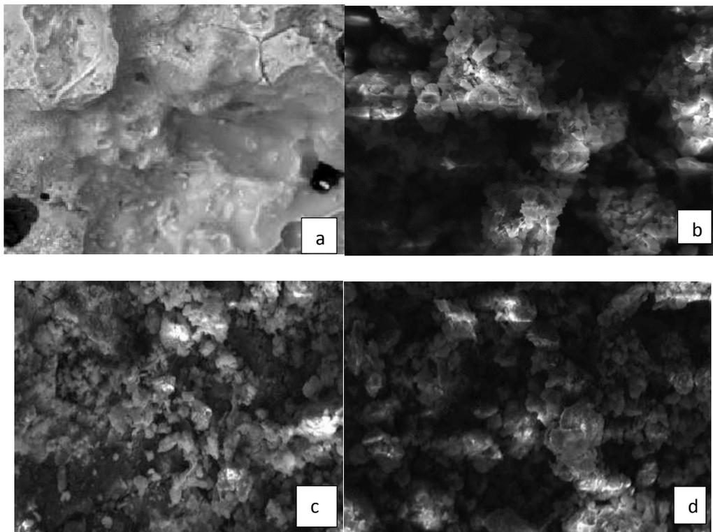
Fig. 3. Morphology a. OPBA pure ,b OPBA with NaOH 2M c .OPBA with NaOH 2,5M d.OPBA with NaOH 3M
